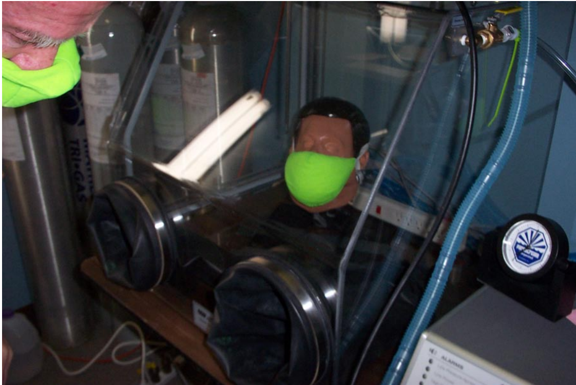
Figure 2. Smoke Mask Mounted on Human Head Simulator Inside Plexiglas Glove Box
