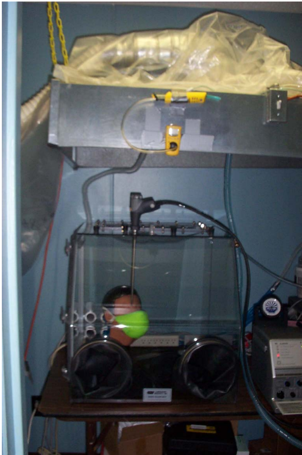
Figure B. Smoke Mask Mounted For Testing On Human Head Simulator In Glove Box
